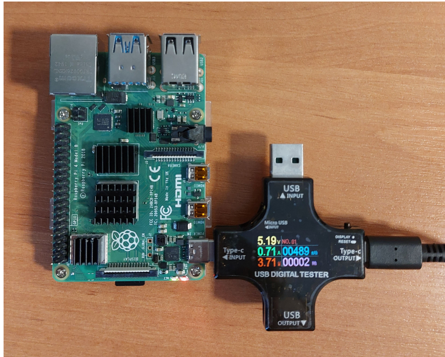
Figure 4.19: Rapsberry Pi 4B with 4GB RAM used for measurements in this section. There is also a USB energy tester connected to power supply, which was used to read power drawn.
