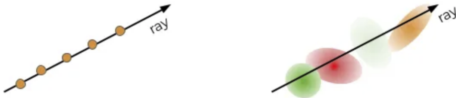
Figure 12: Conceptual difference between NeRF and Gaussian Splatting. Image adapted from [35].
