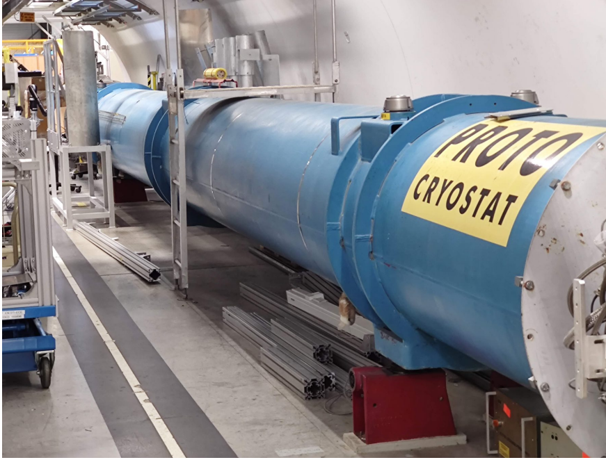
Figure 1.1: Simulation room to replicate the LHC tunnel environment, used for development of robotic systems and for testing their functionality.
