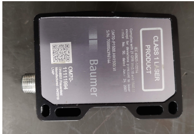
Figure 1.9: Baumer OM70 distance laser used to study remote sensoric detection of respiratory rate.
