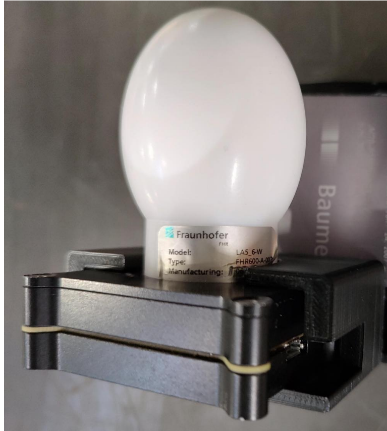
Figure 1.8: FMCW Fraunhofer 80 GHz radar used to study remote sensoric detection of respiratory rate.
