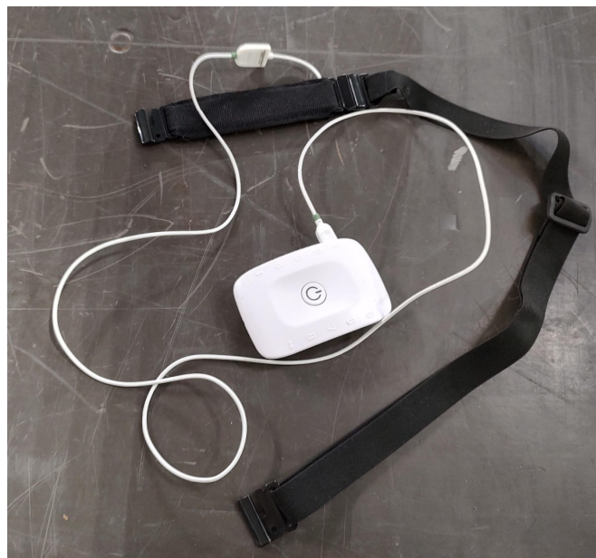
Figure 1.10: PLUX chest belt used to study remote sensoric detection of respiratory rate.
