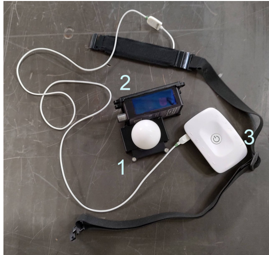
Figure 4.4: Three sensors to detect and calibrate RR: (1) the FMCW Fraunhofer 80 GHz radar, (2) the Bamuer OM70 distance laser, and (3) the PLUX chest belt.
