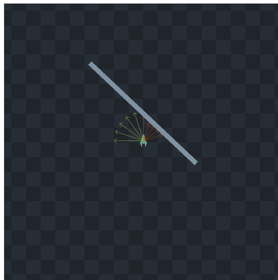
Figure 9.13: Ray casting in a 2D cone, missed rays in yellow, hit rays in red.
