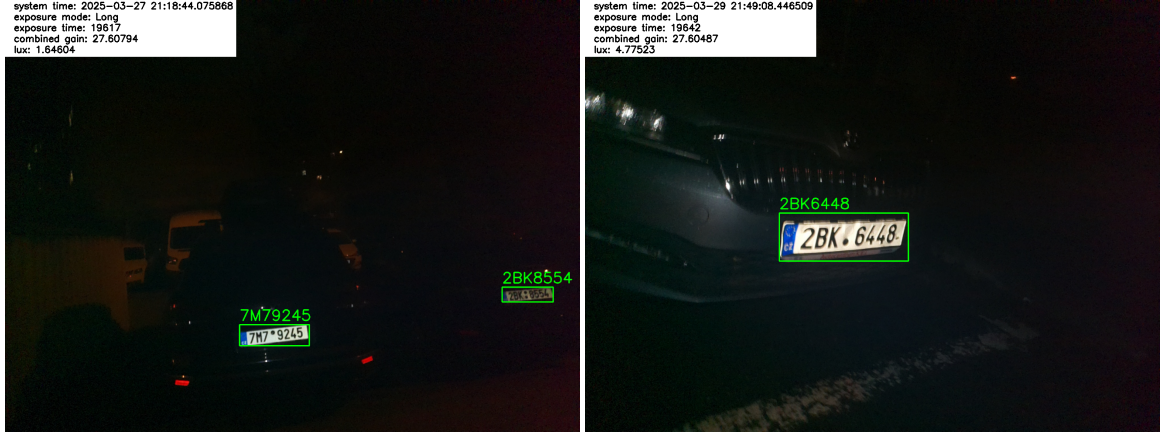
Figure 5.12: Correct night mode registration plate detections and recognition in hand-held footage captured at slow walking speed, see Figure A.10 for more examples
