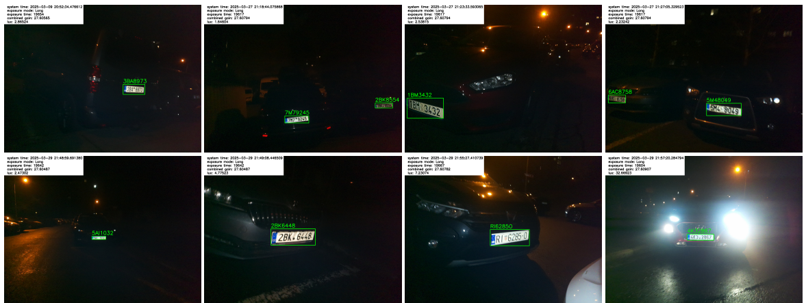
Figure A.10: Correct night mode registration plate detections and recognition in hand-held footage captured at slow walking speed
