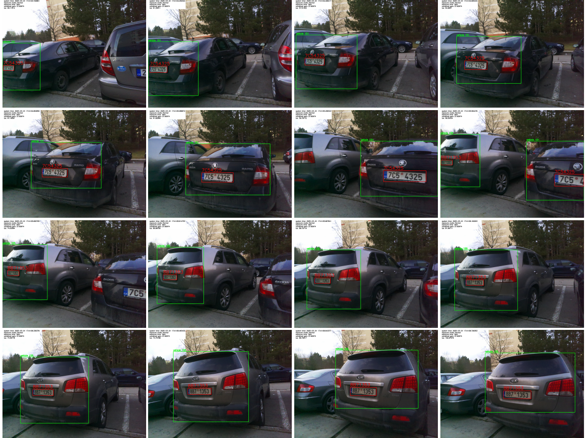
Figure A.2: Correct registration plate readings with configured image signal processing pipeline for shorter exposure times in hand-held footage captured at walking speed
