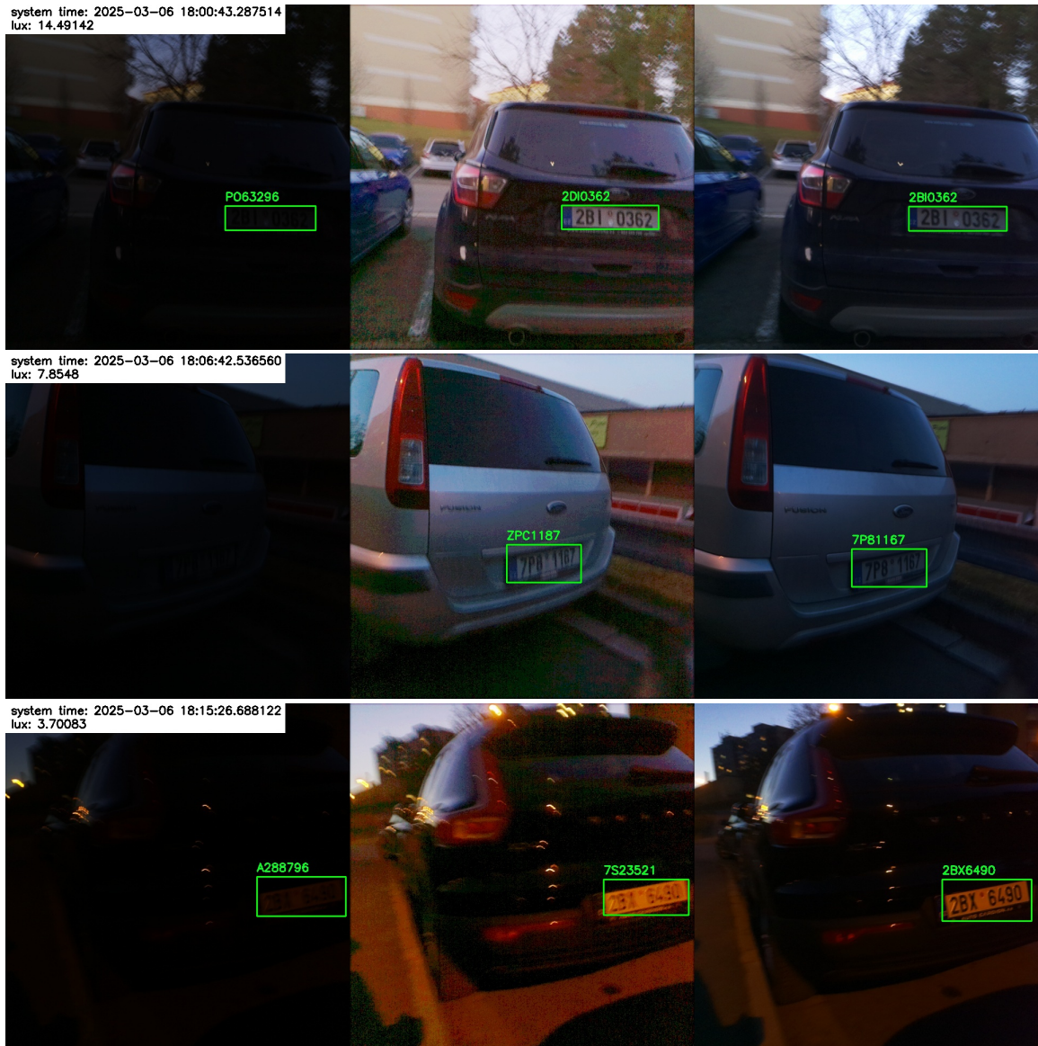
Figure A.8: Correct registration plate readings in long exposure frames (right) during the civil twilight period in hand-held footage captured at slow walking speed
