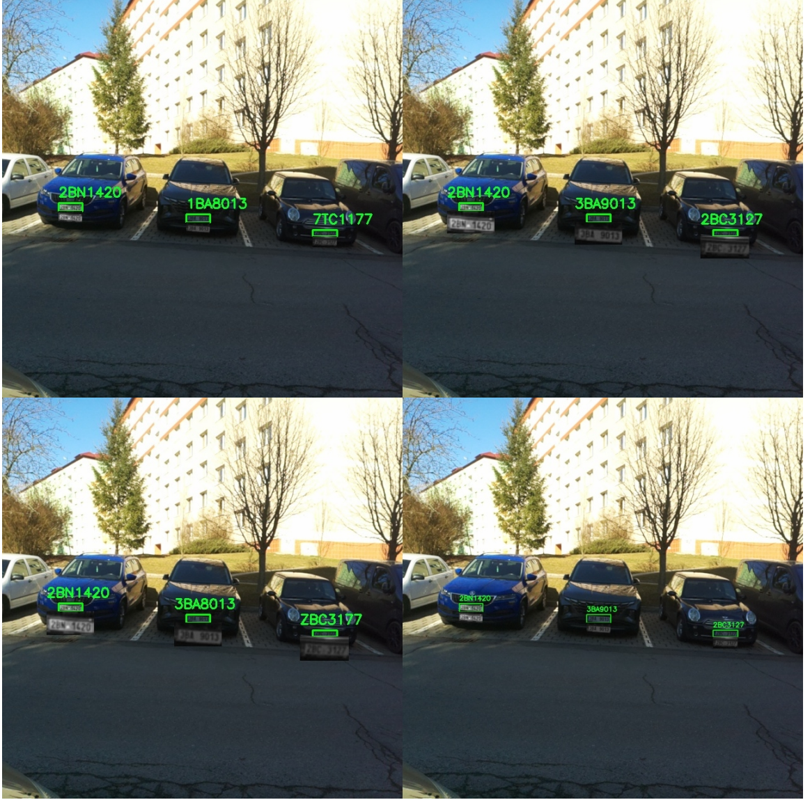
Figure 5.8: Readings of low resolution (left upper), 2x super-resolution (right upper), 2x bicubic interpolation (left lower), and 2x actual crops (right lower) of registration plates across multiple frames in hand-held footage, see Figure A.6 for more examples
