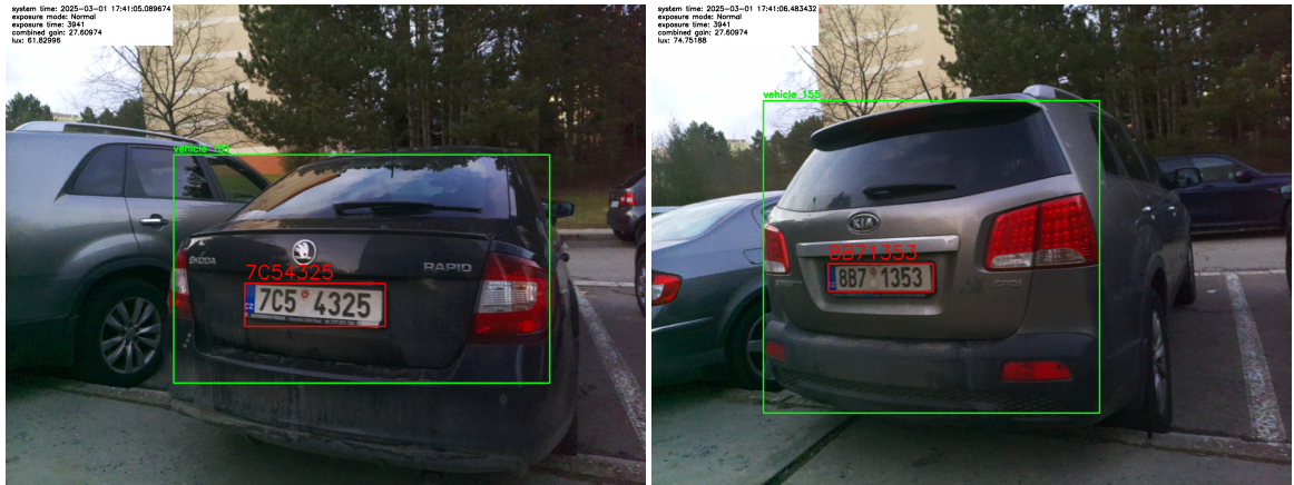
Figure 5.4: Correct registration plate readings with configured image signal processing pipeline for shorter exposure times in hand-held footage captured at walking speed, see Figure A.2 for more examples
