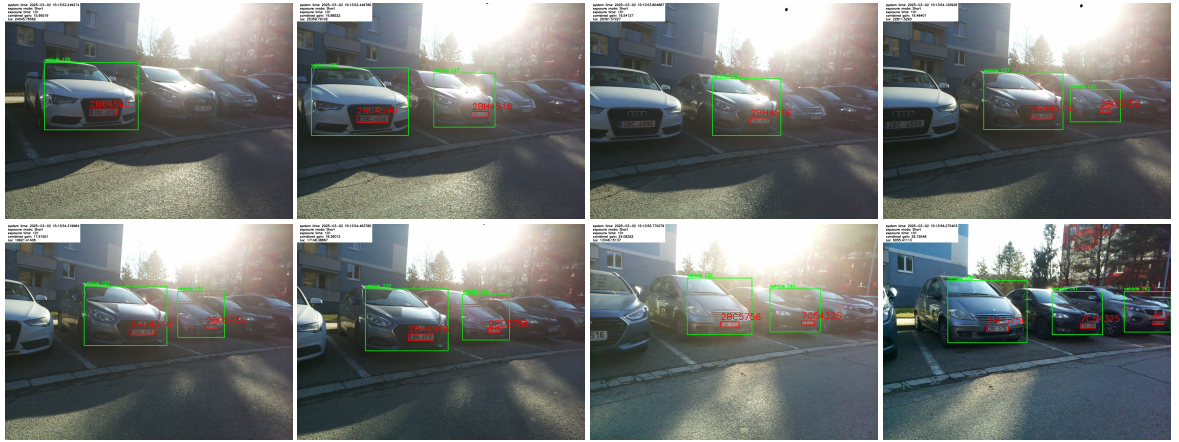
Figure A.5: Fine-tuned vehicle detection model detecting only vehicle fronts, leading to correct registration plate assignment and readings in hand-held footage captured at walking speed
