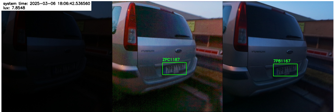
Figure 5.10: Correct registration plate readings in long exposure frames (right) during the civil twilight period in hand-held footage captured at slow walking speed, see Figure A.8 for more examples
