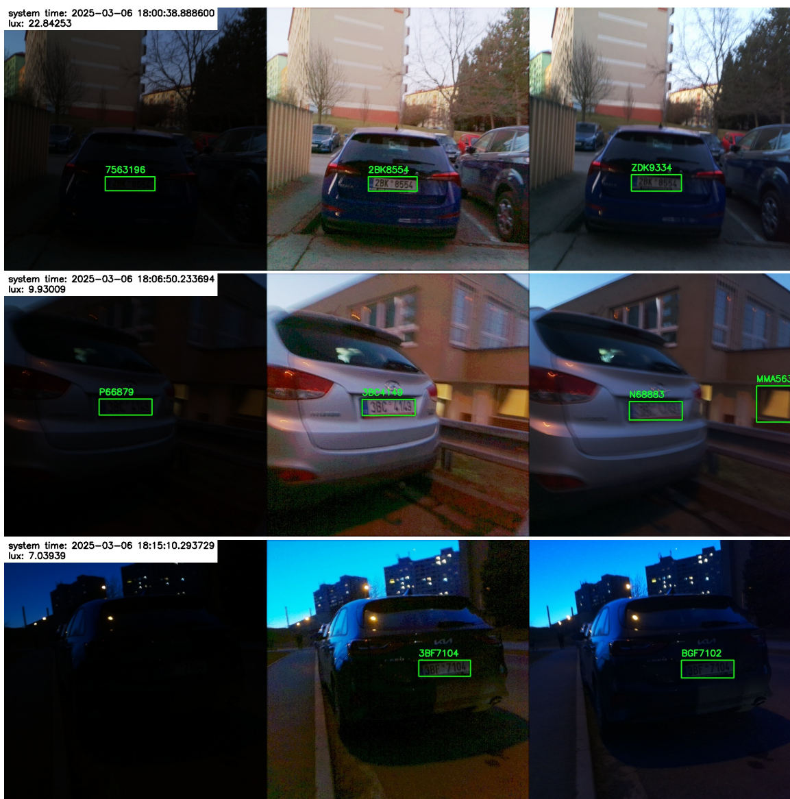
Figure A.7: Correct registration plate readings in enhanced short exposure frames (middle) during the civil twilight period in hand-held footage captured at slow walking speed
