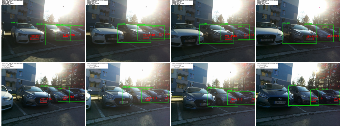
Figure A.4: General vehicle detection model causing overlaps leading to incorrect registration plate assignment, thus their incorrect readings in hand-held footage captured at walking speed
