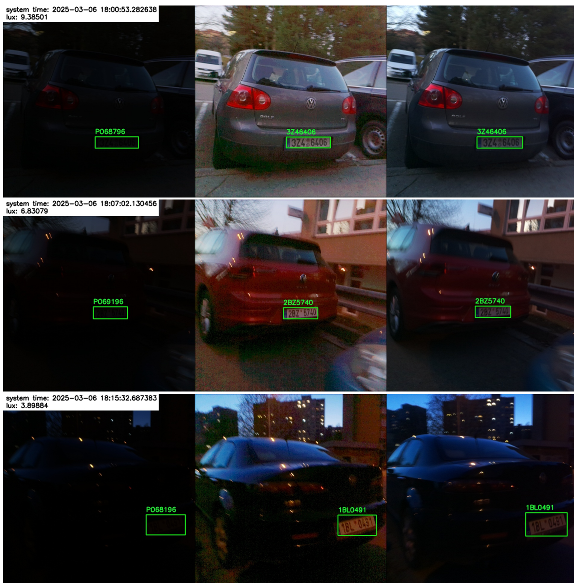
Figure A.9: Correct registration plate readings in both enhanced short exposure (middle) and long exposure frames (right) during the civil twilight period in hand-held footage captured at slow walking speed
