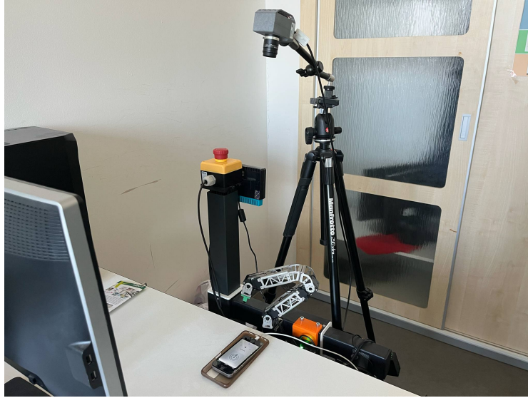
■ Figure 4.1 The AIVA robot setup. The two main components are the robotic arm and a camera.
