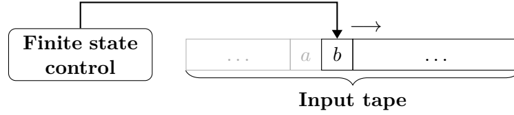
Figure 2.2: General schema of a (one-way) finite automaton.
