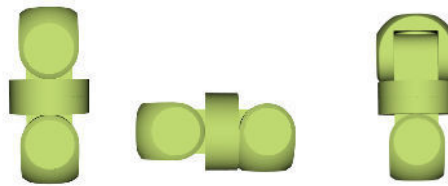
Figure 4.3: Movement of the \alpha joint changes the next body's position, but \gamma doesn't.
