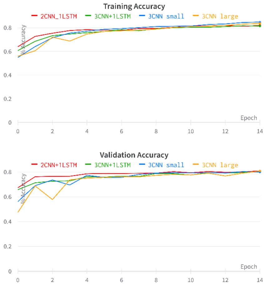
Figure 6.3: [350,700) group training and validation accuracies. The 2CNN+1LSTM architecture is used in the final hyper-tuned model
