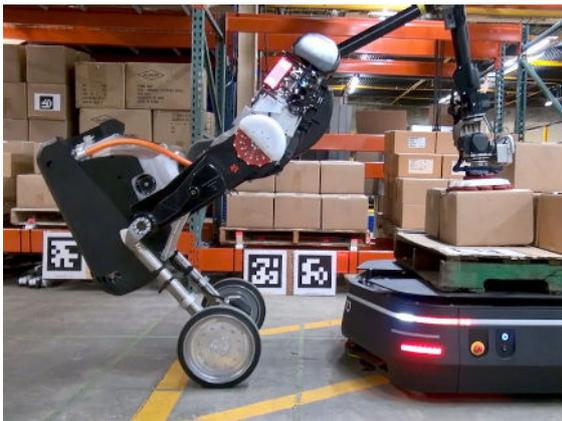
Figure 11: AprilTag markers as labels for warehouse robot [49]
