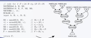
The user describes the mapped function as a sequence of calls to the elementary functions which exchange the intermediate results via off-chip memory. This sequence is then parsed into a data flow DAG with function calls as vertices and data dependencies as edges.
