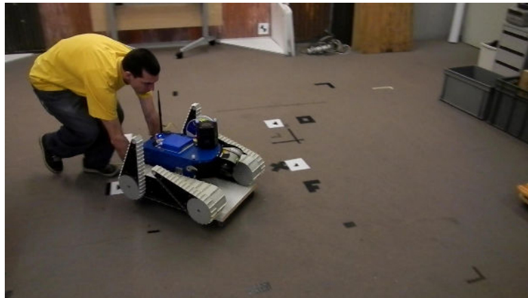
Figure 5.14. There is a trolley beneath the robot, which is pushed forward through the laboratory.
