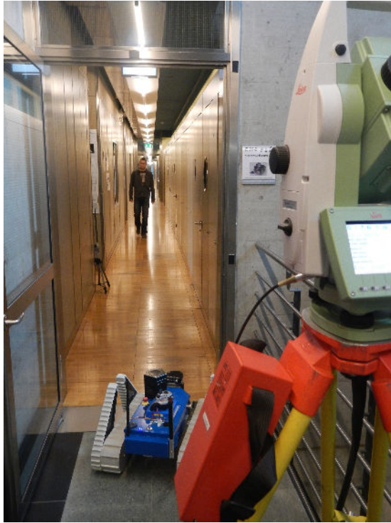
Figure 3.3. The Hallway experiment setup in the Autonomous System Lab, ETH Zürich. This experiment was used to verify or to negate the \beta angle on-the-run estimation, using the Leica TS15 I(1.3) theodolite as a source of reference. The conditions were ideal: 100m long hallway, perfectly leveled.
