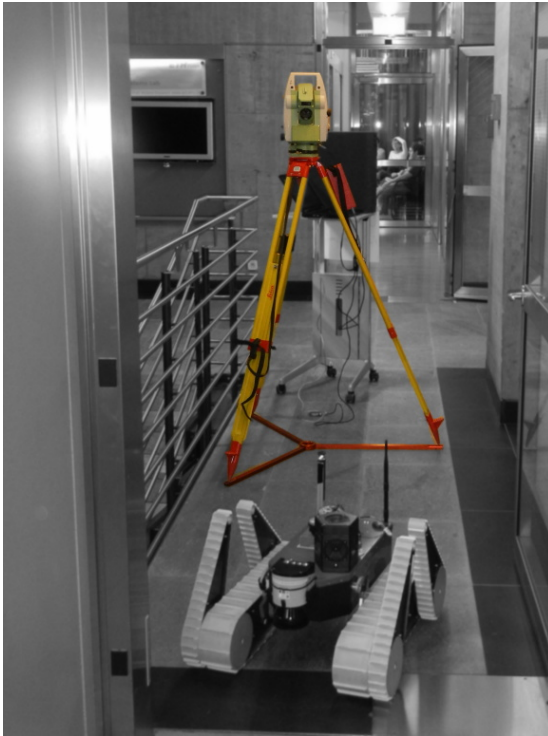
Figure 1.8. The Leica TS15 I theodolite setup during the hallway experiment. It is measuring the distance to the prism attached to the robot with frequency of 15Hz. The measurement is sent to the laptop via a RS-232 link. Similarly to the Vicon system measurements, these are published inside the robot system being labeled with the current robot's system time.
