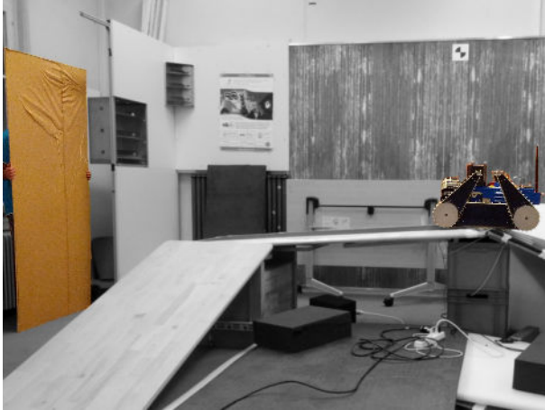
Figure 5.23. The big paper board was held on one spot until the robot reached it and then moved back away from the robot as depicted here. This artificial moving wall confused the ICP localization.
