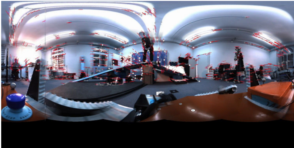
Figure 3.13. Panoramic picture composed of 6 images captured by the Ladybug ® 3 omni-camera in a laboratory of ETH Zürich with correspondences between two consequent panoramic pictures as detected by the visual odometry algorithm implemented by Jiří Diviš for the NIFTi robot. Each red line connects a feature detected in this picture and its new position in the next frame. Directions of the lines indicate that the robot is moving forward. (Color representation is not correct due to the debugging nature of this image)
