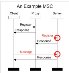
An MSC diagram on which SCStudio finds a race condition: as the communication is asynchronous, the highlighted messages may arrive in any order, where the MSC specifies Message will arrive only after Register.
