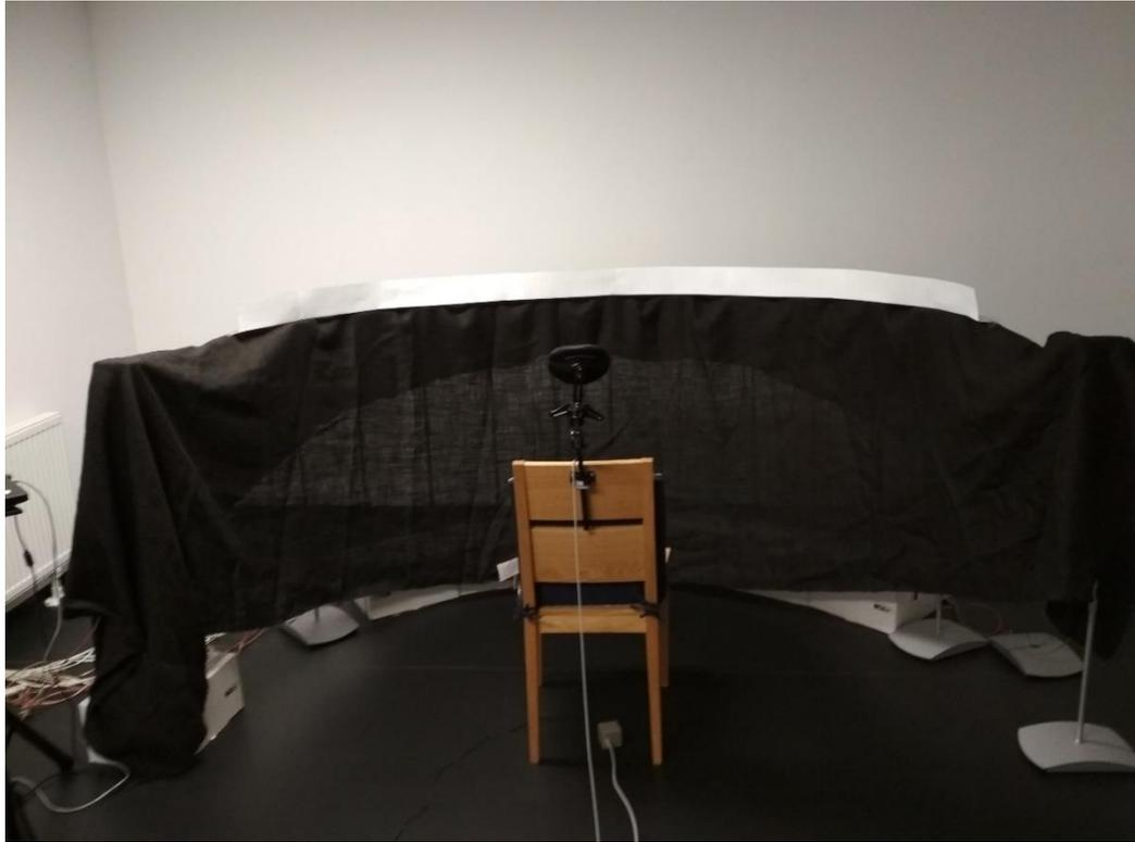
**Figure 2: Room for RE part of the experiment. Chair with the headset is in the middle, loudspeakers are behind black cloth, with white stripe of the paper, for presenting visual stimuli, on the top.**
