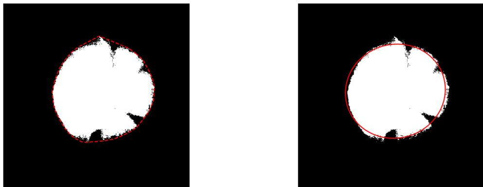
Figure 2.7: The left image shows the convex hull of the object selected by a threshold. The right image shows an ellipse fitted to the boundary of the object selected by a threshold.
