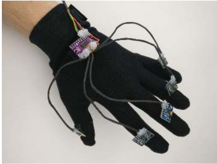
Figure 2.2: Five sensors are attached to the middle phalanges on the fingers and the multiplexer is located in the middle of the back of the hand. All connections are covered with glue for protection and sturdiness.
