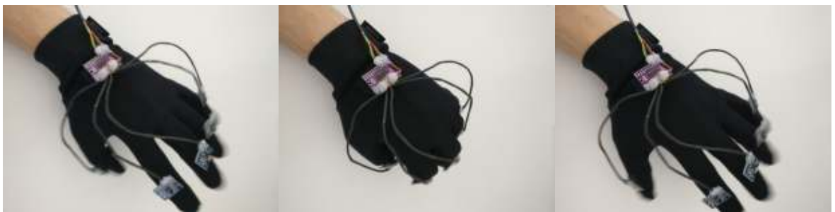
Figure 2.3: Cables leading from the multiplexer to sensors on the fingers are long enough to be non-obtrusive. Performing movements while wearing the glove does not present any major difficulties.
