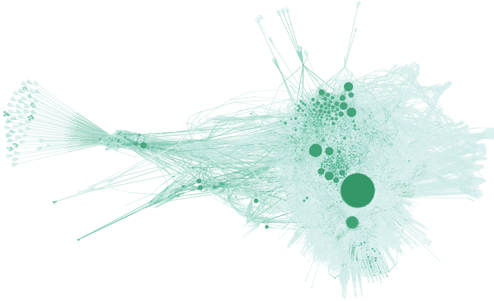
Figure 23: An example of a dependency graph generated by our tool for analysis of the linking process. It shows the HelloWorld application. Nodes represent sections and edges dependencies between them. Size of a node represents the relative size of the section.
