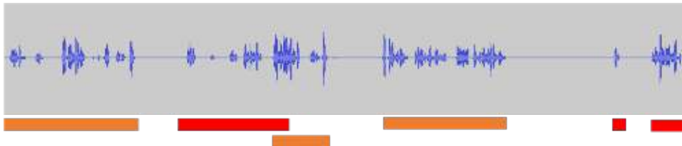
Figure 2.10: Example output of diarization on single channel audio. Different colors in the bottom indicate different speakers.
