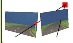
Position is estimated using calculation of intersection of two lines in space, in a way similar to shooting a ray through the optical center of the camera from two different positions in space.
