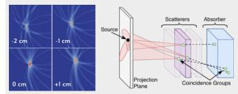
By the Compton equation, each coincidence group defines a conic surface which intersects the unknown  $\gamma\text{-ray}$  source. Triangulating with multiple cones, the source can be accurately localized in 3D space.
