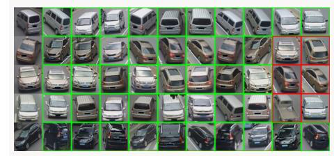
The left column - the query image, the **remaining ten images** are the image representations of the most similar images from gallery. A green border means correctly matched object according to ground truth while a red boarder indicates a different identity from the query.
