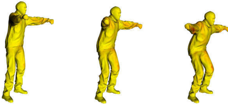
Figure 6.19: Artifacts on the right leg occurring during the whole mesh morphing with Data Dependent Laplacian. Colour visualizes the angle difference from the expected result.
