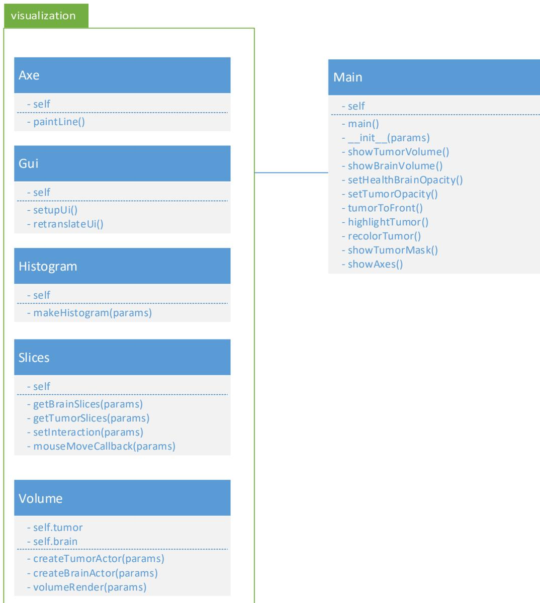
Figure 105: Class diagram of visualization (UML notation)
