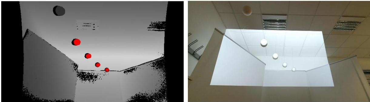
Figure 6-3 Visualization of the homography transformation of the depth map (with ROI locations marked by red colour) to the RGB image space using the inverse homography matrix of the RGB frame projection to the depth point-cloud space. If you place the images one on another, the positions of the pixels would match and refer to the same point in the depth point-cloud space.
