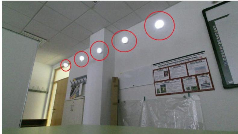
Figure 6-1 Testing the illusion of projecting bright light on specific areas at the scene (marked by red circles) using e.g. theatre reflectors. In fact, LCD projector projects white colour on the ROIs and black colour on non-ROI areas which creates the mentioned illusion.
