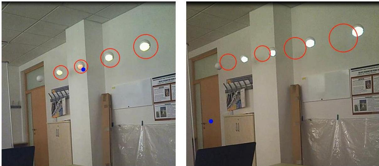
Figure 6-11: Successful tracking of previously segmented ROIs using proposed shift vector computations (left). Tracking error (right) caused by specifics of the egocentric video- constant shakes and fast tilts of the head- and by cumulation of the tracking error. The captures are from the prototyping phase of the module proposal.
