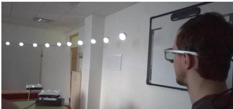
Figure 5-2: Participant, ready to start an experiment, captured along with the complete scene setup with desired projection on the ROIs. The eye tracker is mounted to a computer with running data acquisition module.
