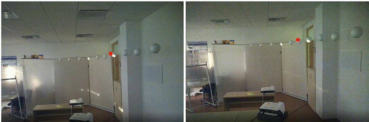
Figure 7-6 Captures of the egocentric video frames (with gaze written in as a red dot) at the same moment during the experiments with two different participants. The capture on the left side visualizes decent quality of the obtained gaze data while the capture on the right side visualizes bad quality of the gaze data. Both participants are looking at the closer ROI with projected face.
