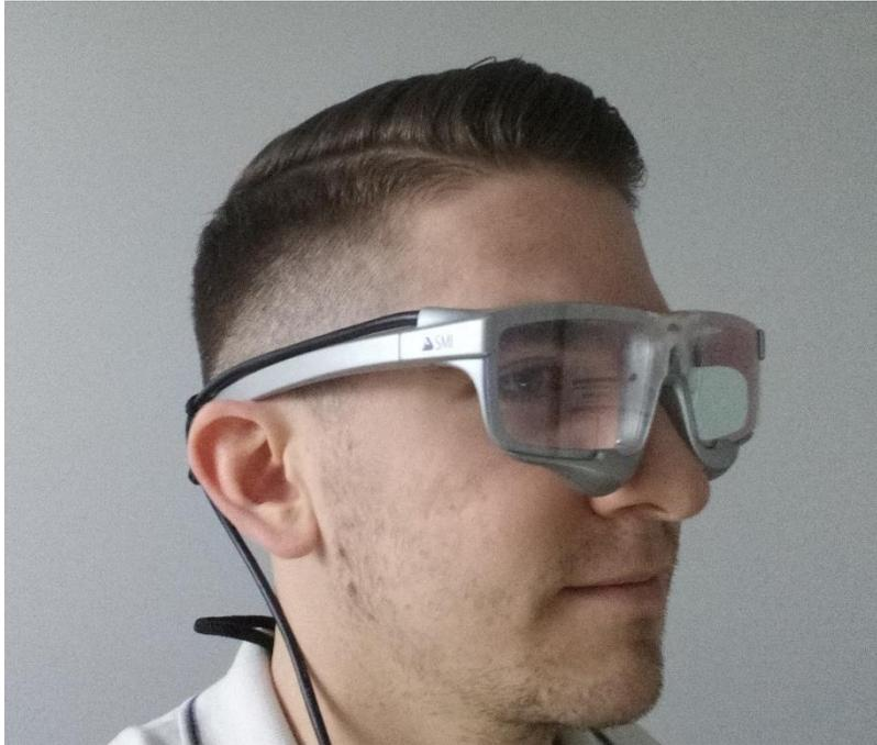
Figure 6-8: The observer equipped with the mobile SMI Eye Tracking Glasses. The eye-tracker is connected through the cable to a computer with the running eye-tracking module.
