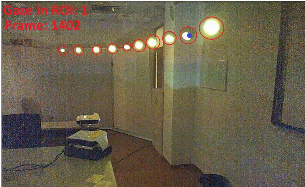
Figure 6-12 Automatically evaluated egocentric video frame from the dataset by the automatic evaluation module (graphic output). Tracked ROIs are in red circles (they have enlarged areas) and gaze is a blue dot. The intersection is displayed in the top-left corner. ROIs are numbered from the right-hand-side starting from the zero.
