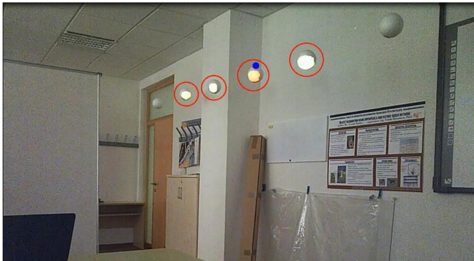
Figure 7-5: Partial solution for the eye-tracker's gaze error which was additionally proposed and implemented in the automatic evaluation module. The ROI areas (red circles) are enlarged when searching for the gaze-ROI intersection by the evaluation algorithm.
