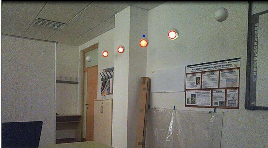
Figure 7-3: Gaze error from the eye-tracker after its proper calibration. The error is unpredictable (as stated on Figure 7-1), and its causes are not clear, yet. However, the eye-tracking hardware is significantly out-dated, nowadays.
