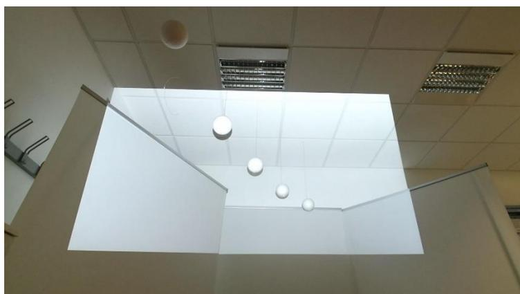
Figure 6-2 The RGB frame from the Kinect with the visible projection plane that can be easily segmented from the frame. Projection of plain white colour during the calibration is handled by the calibration module.
