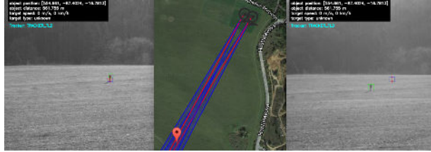
Figure 8. The two-camera setup, where a distant target is tracked by both CSs (left and right). The estimated position of the target is displayed in the map (center) in real time.
