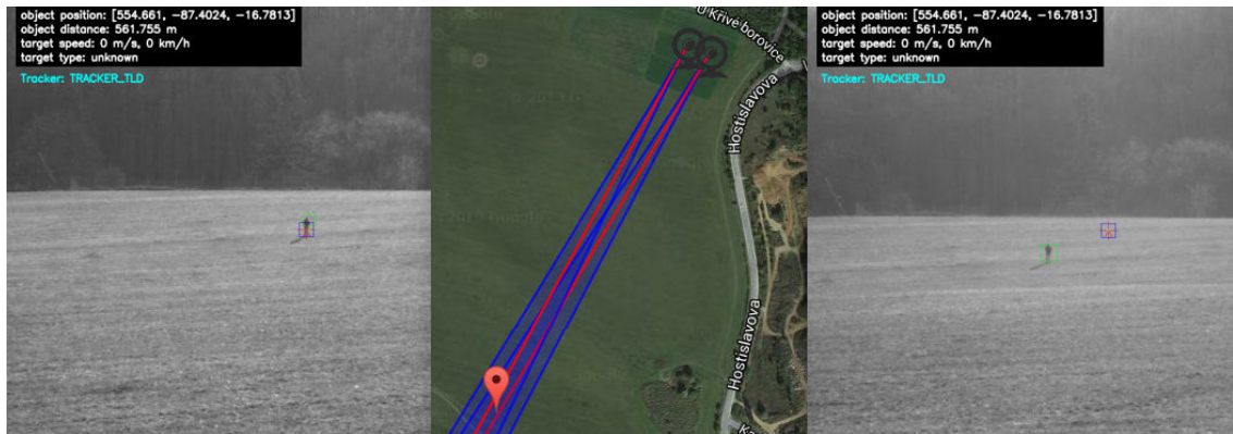
Figure 6.6: The two-camera setup where the distant target is tracked by both CUs (left and right). The estimated position of the target is displayed in the map (center).
