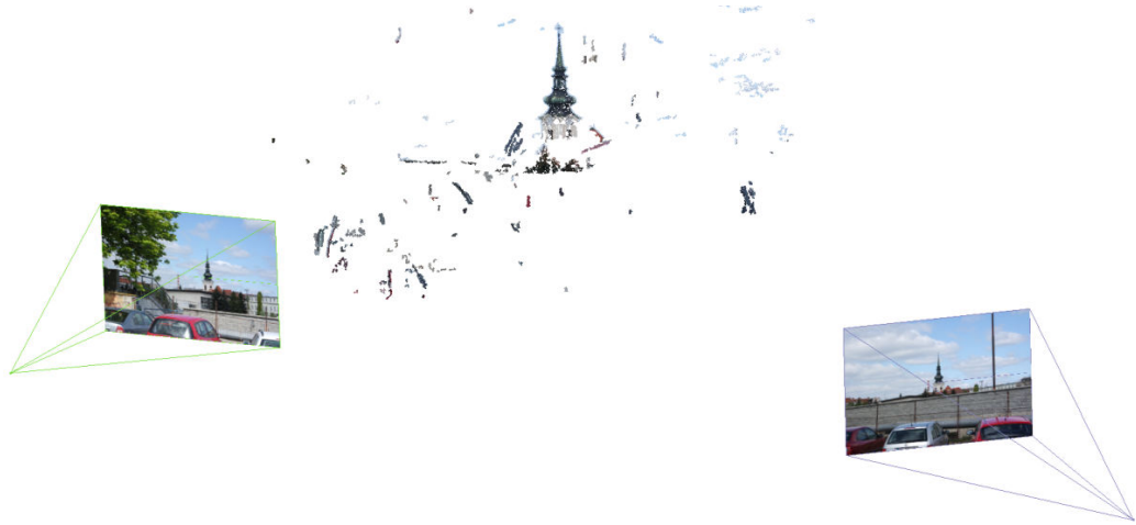
Figure 2.12: 3D reconstruction performed by VisualSFM from only two photographs taken by the same camera in district Štýřice (Brno, Czech Republic). Note that even mere two views suffice to reconstruct the church tower, however, the output data include a lot of noise.
