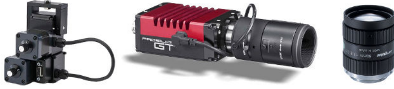
Figure 4.2: Product pictures of P&T unit Flir PTU D46-70 (left), camera Prosilica GT 1290C (middle) and lens Computar M5018-MP2 (right).
