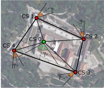
This poster presents a semi-autonomous multi-camera system for **tracking and localizing** the **distant objects**, which is based merely on ordinary RGB cameras. As opposed to the ubiquitous radar based solutions, this system is passive (the target is unaware that it is being tracked) and highly portable which allows fast deployment in various scenarios such as perimeter monitoring or **early threat detection** in defense systems or **air traffic control** in public space.
