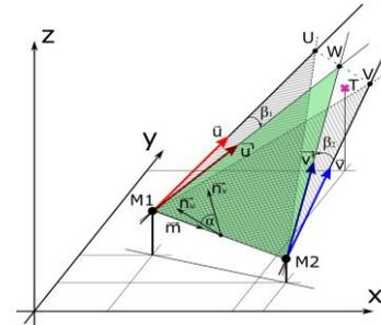
The estimation of the target location is based on multi-view triangulation working with noisy measurements. The **back-projection** is used to find the direction vectors. Target location is estimated as the weighted centroid of the estimates computed by each pair of the camera and with respect to the local **geometry constraints** and **tracker confidence**.
