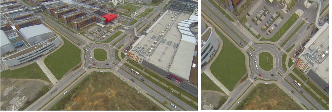
Figure 3.5: Geo-registration of the input video frame. Left: before the transformation into real world coordinate system. Right: after the transformation into real world coordinate system. Note that the vehicles at the top of the untransformed frame (left) are considerably smaller — this size distortion is caused by perspective effect: farther objects appear to be smaller. In the geo-registered frame (right), such effect is not present.
