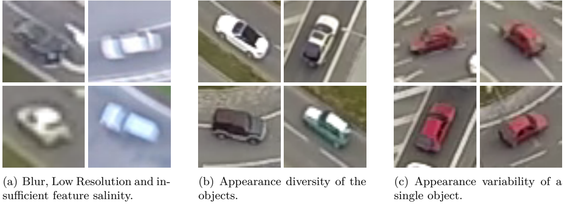
Figure 4.3: Characteristic problems of vehicle representation in aerial video data. All images are extracted from evaluation datasets (see section 8.1).
