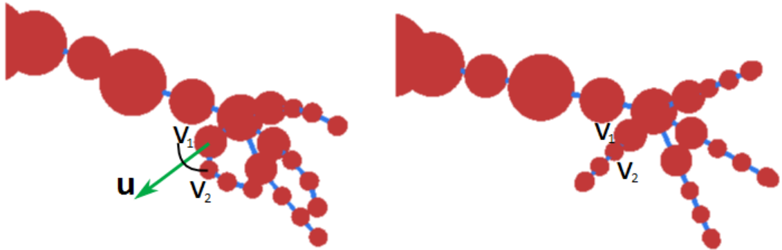
Figure 2.1: Skeleton straightening. Left: input skeleton, green arrow represents the direction from connection nodes parents position to connection nodes position, black curve marks the distance between connection node and its child; right: straightened skeleton.
