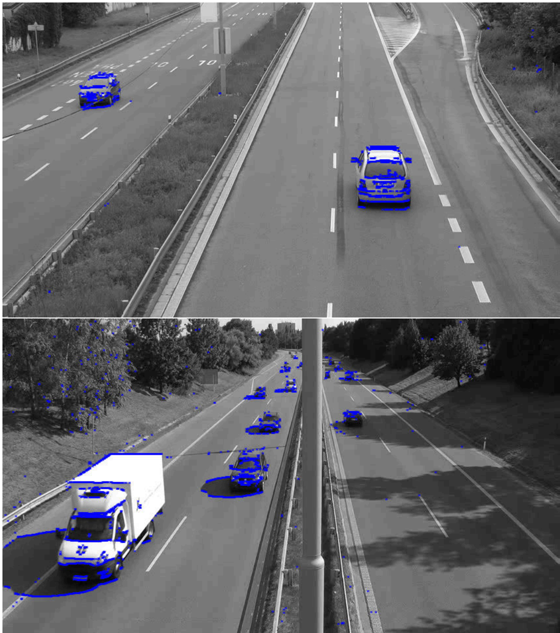
Figure 4.4: Examples of points which define lines which are accumulated into the diamond space for the second vanishing point detection.
