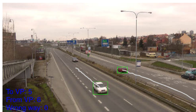
Figure 1: Example of video scene processed by the proposed traffic analysis system. Information about passing cars and their directions are displayed in output video.
