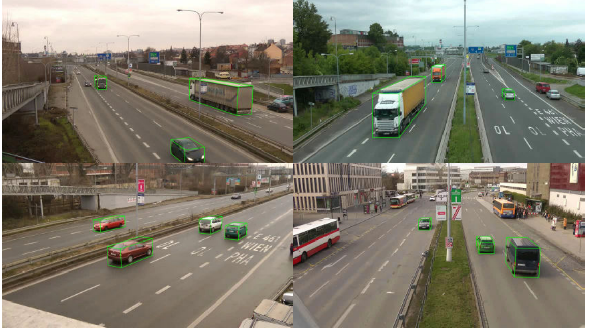
Figure 4.12: Examples of detected three-dimensional bounding boxes for different scenes.
