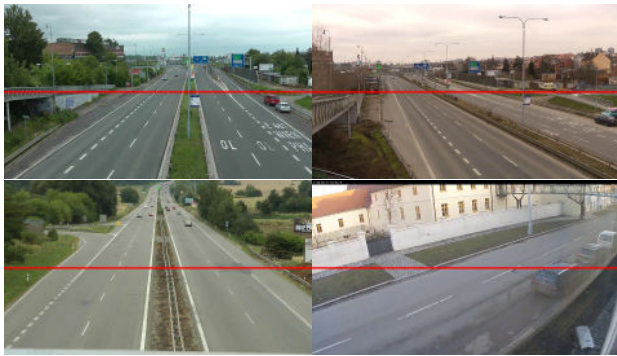
Figure 8: Examples of videos for detection and tracking evaluation. Virtual line which was used for manual ground truth annotation is drawn by red color.
