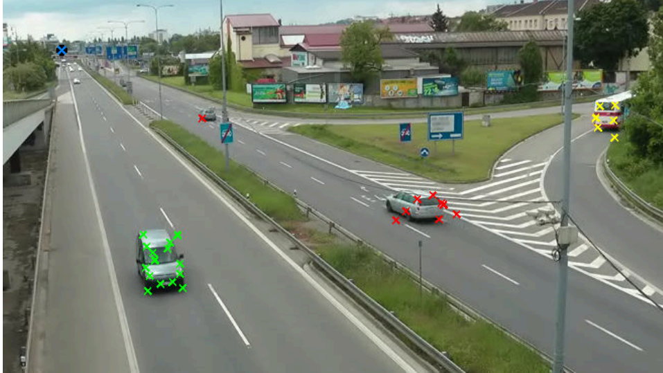
Fig. 3. Tracked points and their classification based on the first VP position. Points marked by red/green move towards/from the first VP. Points marked by yellow are moving elsewhere.
