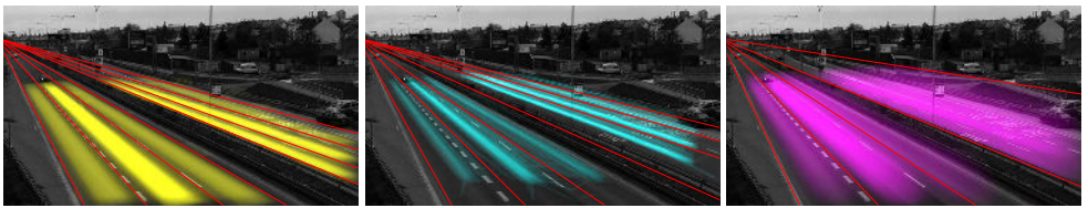
Figure 8: Traffic lane segmentation. ( left ) Our approach based on 3D bounding boxes. Lanes are correctly segmented even for side views. ( middle ) Method using trajectories of the centers of blobs [16]. ( right ) Method based on activity map [28].
