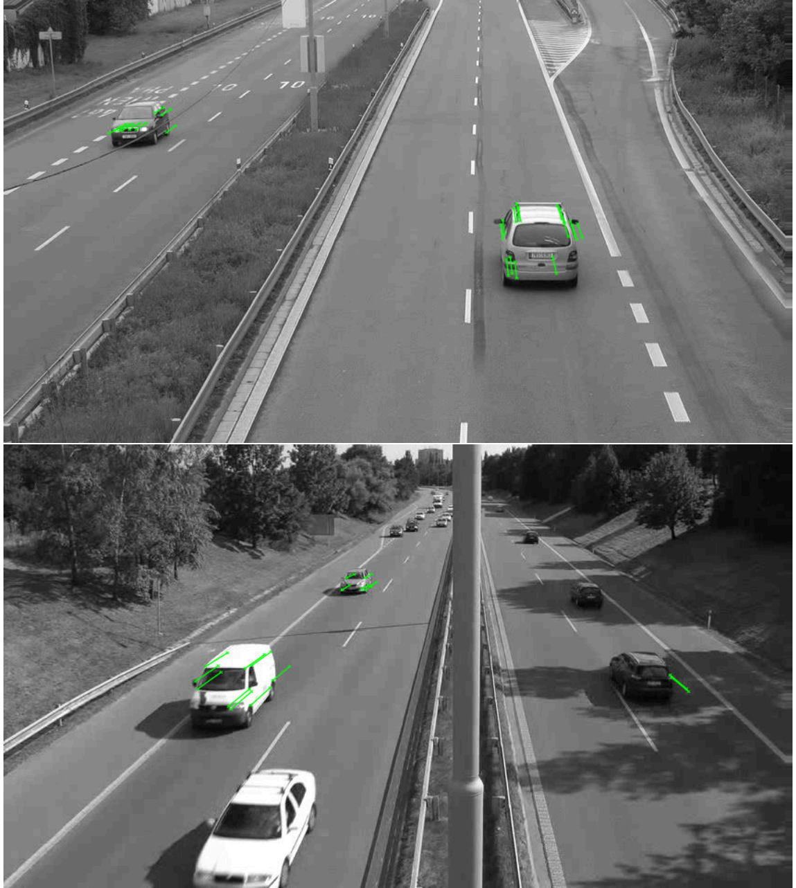
Figure 4.3: Detected and tracked corner features for the first vanishing point detection.
