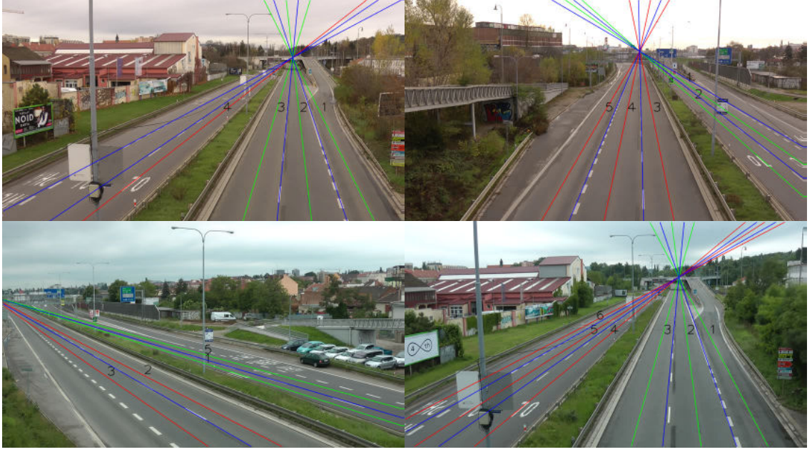
Figure 6.6: Detected lanes (green, red) and lane-dividing lines (blue). As it is shown, the lanes and lane-dividing lines are detected with a high accuracy even for distant lanes and lane-dividing lines.
