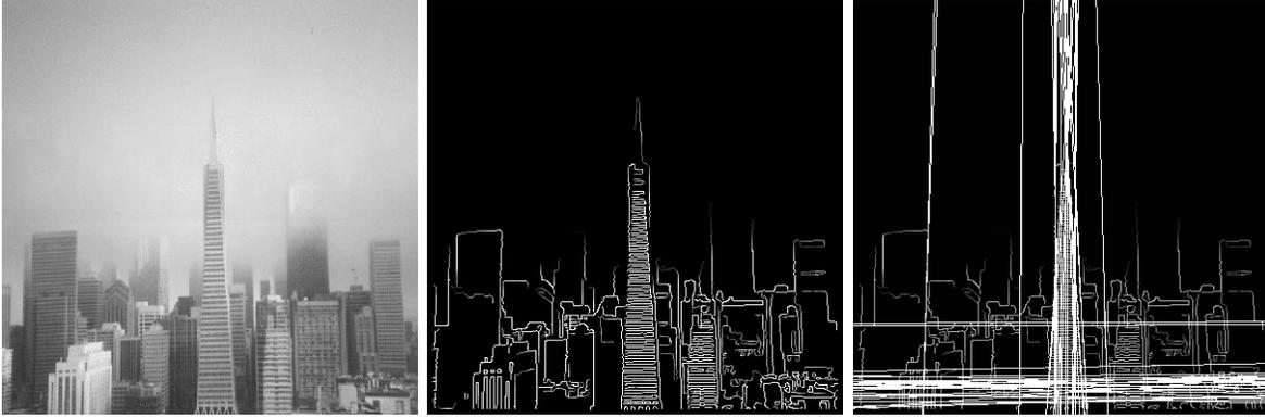
Figure 15: From left to right: original image from Robert Fisher (Fisher, 2003), edges from Canny edge detection applied to the original image, edges overlaid with lines identified by Hough transformation.
