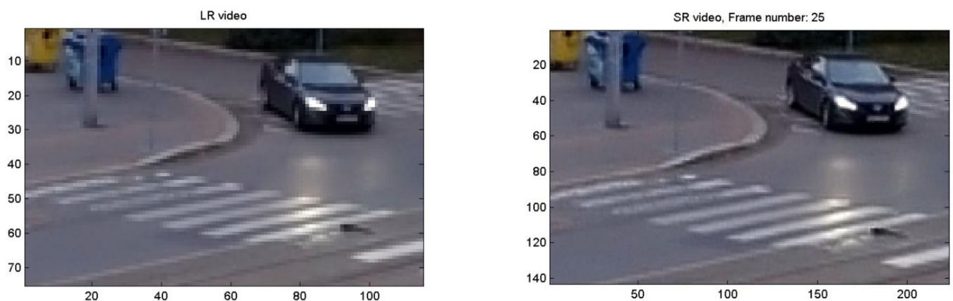
Figure 20: Frame 25 of the Corner video sequence,  $srFactor = 2$ , *optFlow\_LK\_pyramid* motion estimation, *interp\_Delaunay\_bicubic* interpolation
