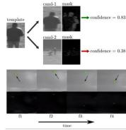
The tracking is based on two state-of-the-art approaches. TLD tracker leverages **detection and tracking** and it is robust against appearance change. The BGFG tracker combines the BG subtraction, motion model and object model in the **bootstrap particle filter framework**. Each measurement is assigned a confidence, localization subsystem can thus combine the measurements in the weighted manner.
