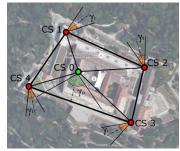
This poster presents a semi-autonomous multi-camera system for tracking and localizing the distant objects, which is based merely on ordinary RGB cameras. As opposed to the ubiquitous radar based solutions, this system is passive (the target is unaware that it is being tracked) and highly portable which allows fast deployment in various scenarios such as perimeter monitoring or early threat detection in defense systems or air traffic control in public space.
